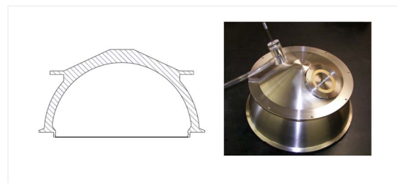
Fig.10 The Nereus main housing end cap with vacuum port sealing assembly
